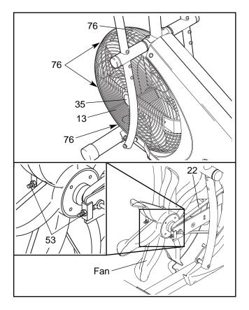
If the Belt (22) needs to be adjusted, loosen the right Guard Fastener (not shown). To tighten the Belt, turn the M6 Nuts (53) clockwise; to loosen the Belt, turn
